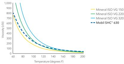
Mobil SHC™ 600 Series lubricants run 20% cooler than conventional oil
