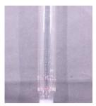
The Mobil DTE™ FM Excel Series shows excellent resistance to oxidation and deposit formation. In the CEC L-48-00-B Oxidation Test (192hrs, 120 °C, air I/h) the oil remains clear, with no visible signs of darkening or deposits.
